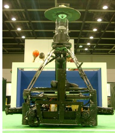
**Figure 3.** Tribot, omni-directional drive and camera
