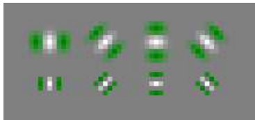
Fig. 3. The four kernels used for the detection of oriented line segments in two different sizes.
