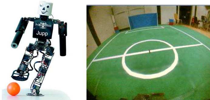
Fig. 1. The left image shows one of our humanoid robots. The robot is controlled by a Pocket PC and uses the images of a low-cost wide-angle camera for perceiving the relevant information about the environment. An image captured from the robot's perspective while it was walking can be seen on the right.
