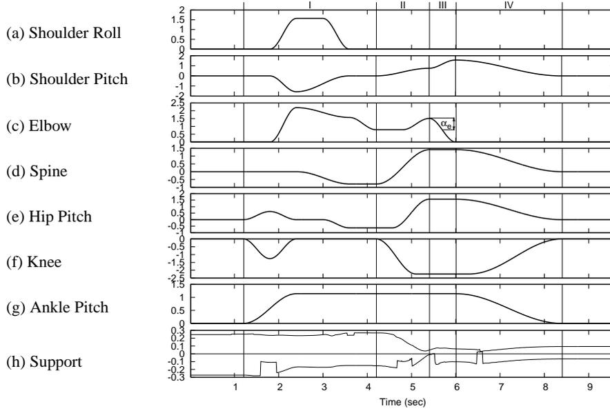
**Figure 5.** (a)-(g) Target positions (in rad) of individual joints when standing up from the prone posture ( $\alpha_e = 0.24\pi$ ). (h) Distance (in m) of the COM projection to the extreme points of the support polygon in sagittal direction.
