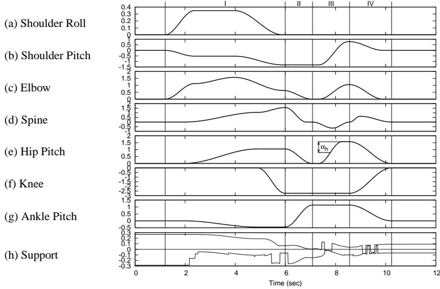
**Figure 3.** (a)-(g) Target positions (in rad) of individual joints when standing up from the supine posture ( $\alpha_h = 0.25\pi$ ). (h) Distance (in m) of the COM projection to the extreme points of the support polygon in sagittal direction.
