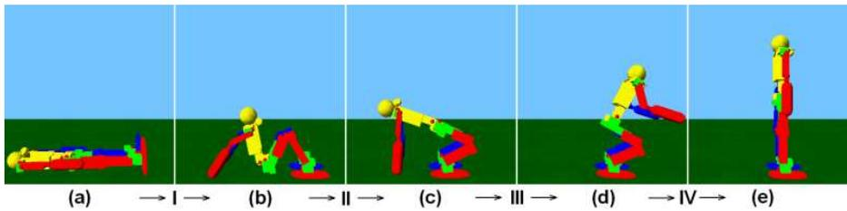
**Figure 2.** (a)-(e) Starting and end positions of phases I-IV when standing up from the supine posture.
