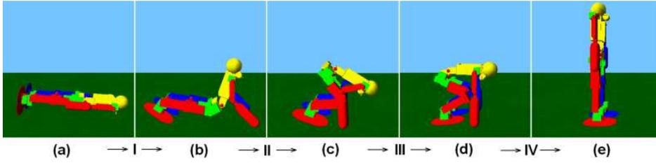
**Figure 4.** (a)-(e) Starting and end positions of phases I-IV when standing up from the prone posture.
