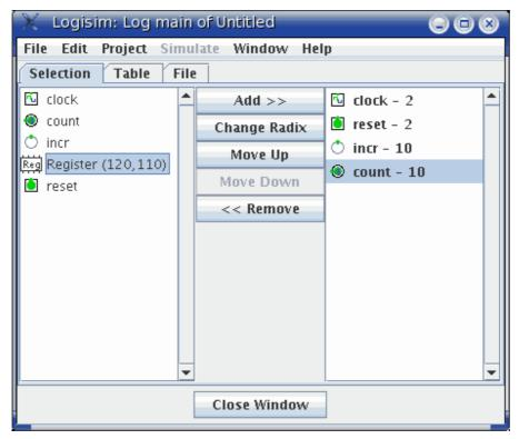
The tab is divided into three vertical areas. The first (leftmost) is a list of all components in the circuit whose values can be logged. Among the built-in libraries, the following types of components support logging.
