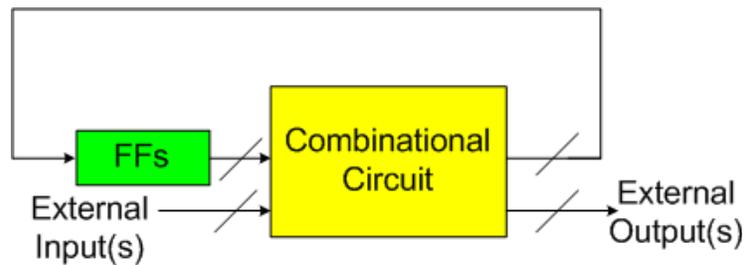
Since ROM can implement combinational logic, so this part can be replaced by a ROM and Flip-Flops can be replaced by a register as shown in the figure.
