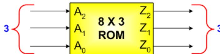
The ROM table is identical to the state transition table with **Present State** and **Inputs** specifying the **address** of ROM and **Next State** and **Outputs** specifying the ROM **outputs (stored information)**. It is shown below:
