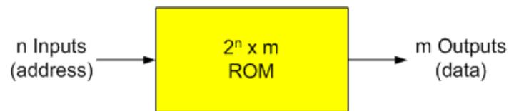
Like RAMs, a ROM has  $n$  address inputs and  $m$  outputs. This corresponds to  $2^n$  memory words each of  $m$  storage bits for a total capacity of  $2^n \times m$  bits.
