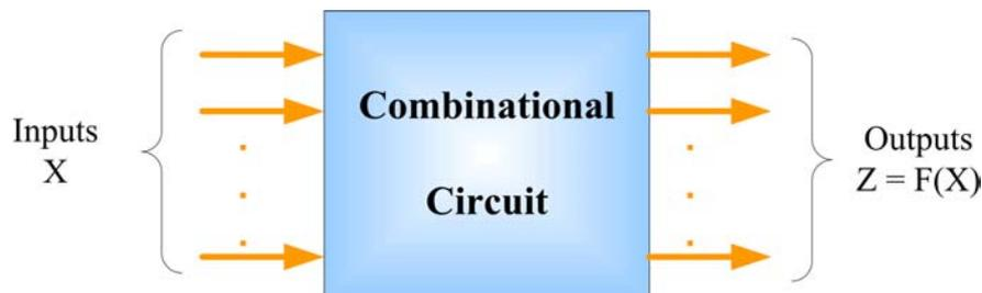
Figure 1: General Block Diagram of a Combinational Circuit
