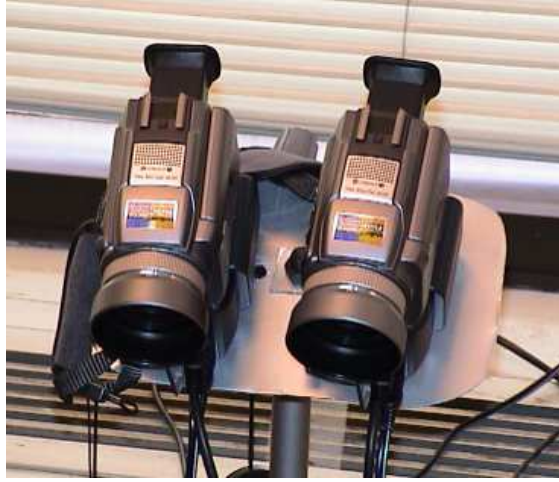
Figure 6: Two digital cameras mounted on an aluminum platform. A single tripod is holding the platform,
