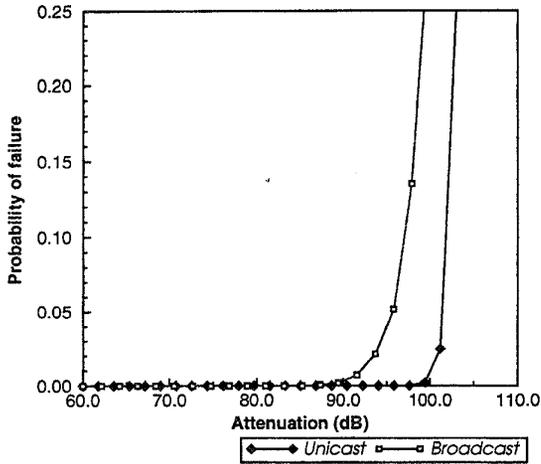
This confirms the analysis of section II.A. Retransmission, as any diversity technique, allows a gain of a few dB in the usable attenuation, adding in this case nearly 10 dB of attenuation to unicast packets compared to broadcast packets (however, unicast transmissions need a much better reliability than broadcast).
