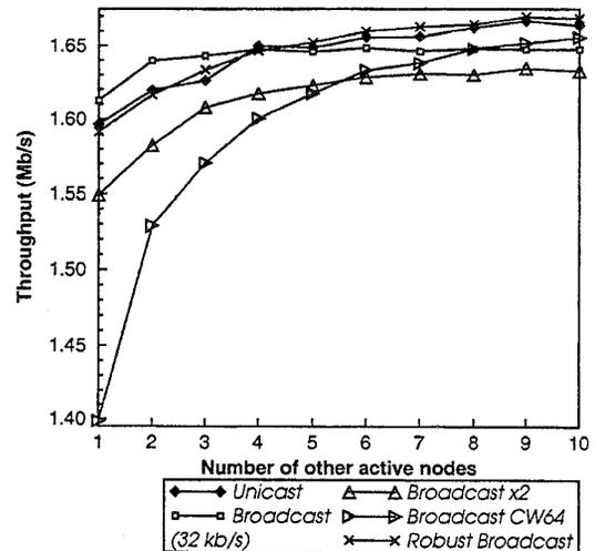
To analyse how those results scale with a different traffic, the same simulations have been performed with the throughput of the broadcast node being 128 kb/s instead of 32 kb/s (quadruple the size of each broadcast packet). The results are shown in Figure 6 (the failure rates in this case are the same as in Figure 4).
