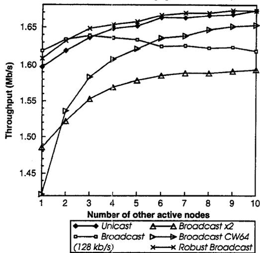
Duplicating each broadcast message ( $\times 2$ ) reduces the available network throughput by the amount of information duplicated (in this case, 32 kb/s or 128 kb/s, plus the overhead, minus the packets discarded due to timeout). Increasing the contention window to 64 ( $CW_{64}$ ) has also a significant impact on the network performance, especially for small number of contending nodes.
