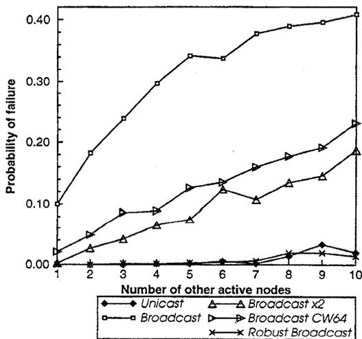
The network is composed of one broadcast (or unicast) node loaded with a voice traffic and an increasing number of unicast nodes (using the data traffic model) contending for the medium. Figure 4 shows the packet failure rate of these different solutions. As we measure only the packet failure rate, these results are quite independent of the traffic nature (arrival rate, packet size...).
