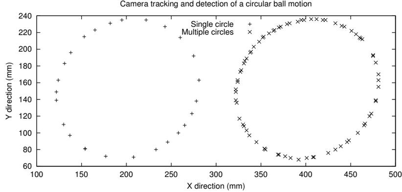
Figure 6: Tracing of the detected motion of a red ball held by a moving robot
