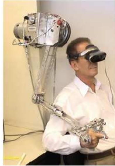
Fig. 2. Master arm station: a user wearing a Head-Mounted Display (stereo vision) and tele-operating using a 6 dof anthropomorphic master arm for motion rendering and force display
