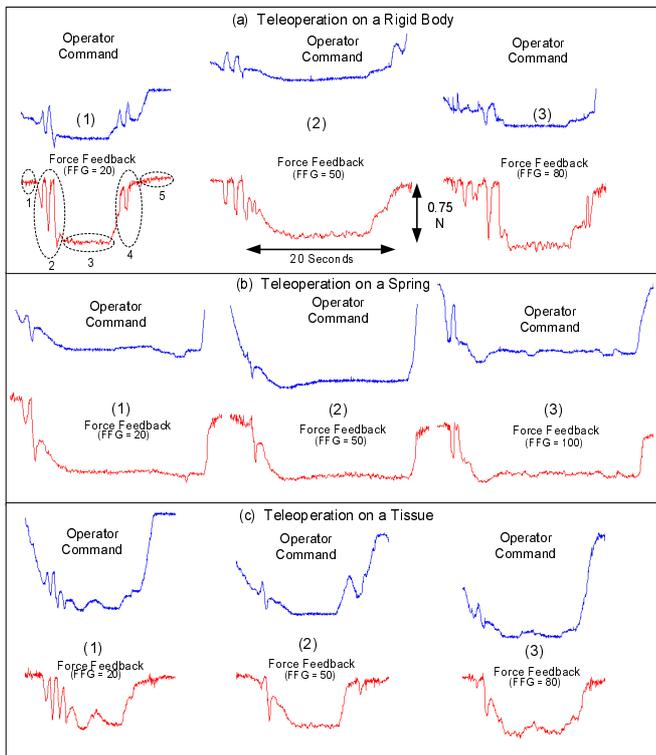
Fig. 3. Operator commands and force feedback during contact with a rigid body (a), a spring (b), and a tissue (c)
