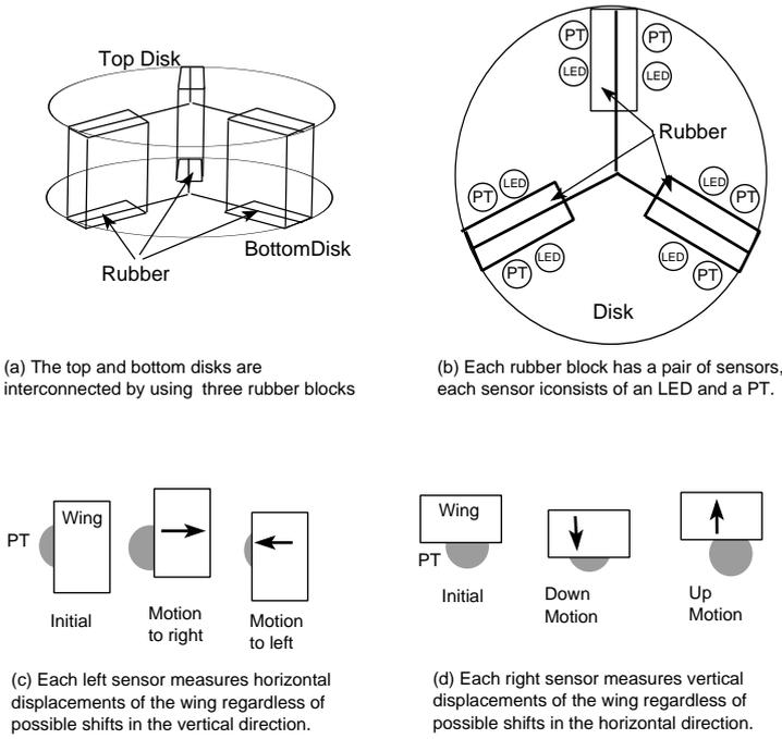
Fig. 2. Some details of the compliant force sensor
