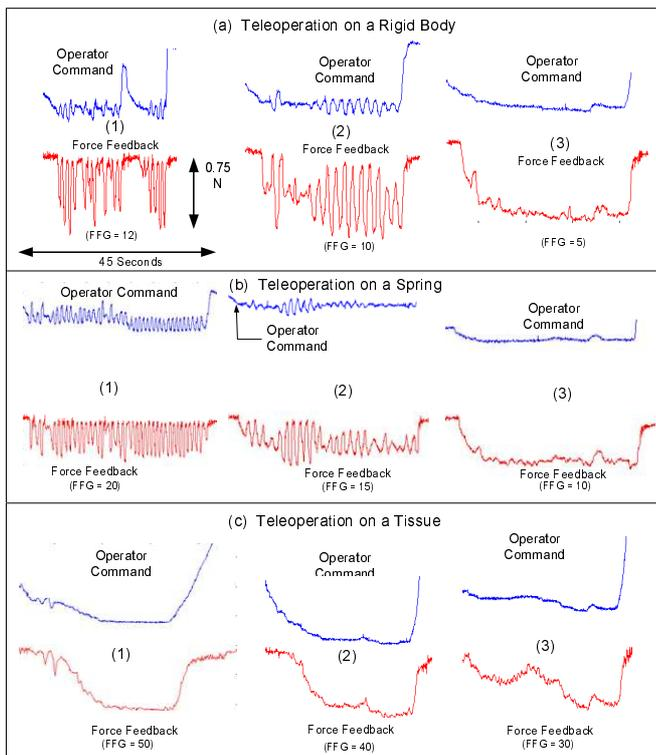
Fig. 4. Extended command-force interactions of pre-contact for a rigid body (a), a spring (b), and a tissue (c)
