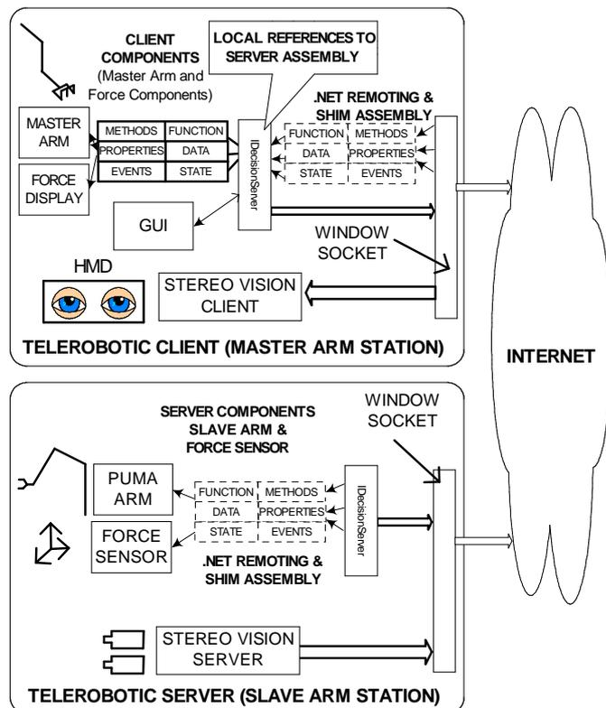
Fig. 1. Real-time transfer of motion command, force data, and live stereo video.
