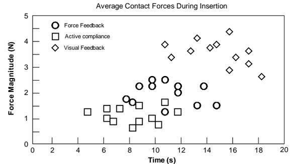
Fig. 9. Average insertion forces with respective task times
