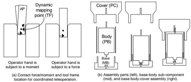
Fig. 4. Strategy used for peg-in-hole insertion and assembly of a water pump.
