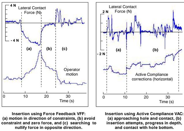
Fig. 5. Insertion using force feedback (a) and active compliance (b).
