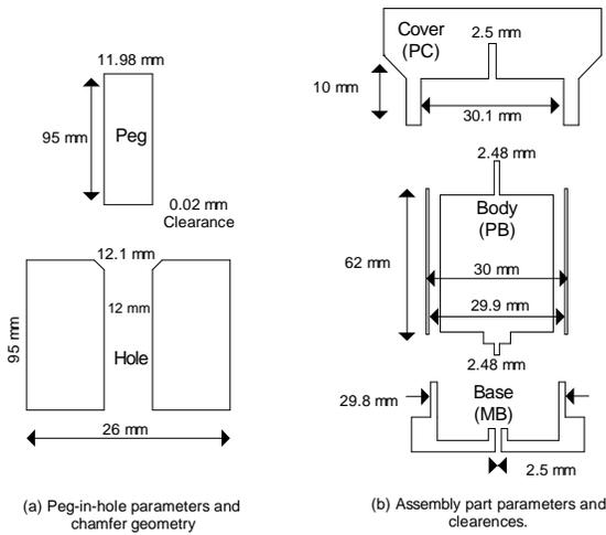
Fig. 2. Features and parameters of the peg-in-hole and pump components
