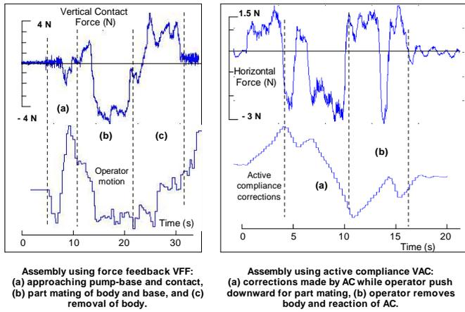
Fig. 6. Assembly using force feedback (a) and active compliance (b).
