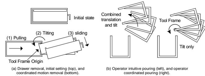
Fig. 7. Strategy used for operating a drawer and pouring water
