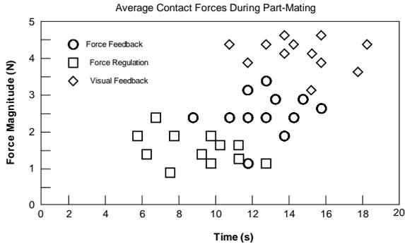
Fig. 11. Average assembly forces with respective task times
