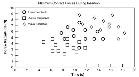
Fig. 8. Maximum insertion forces with respective task times
