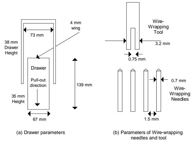
Fig. 3. Dimensioning parameters of drawers and wire-wrapping experiments
