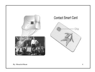
A **contact less card** requires only close proximity to a reader. Both the reader and the card have antenna and it is via this contact less link that the two communicate. Most contact less cards also derive the internal chip power source from this electromagnetic signal. The range is typically two to three inches for non-battery powered cards, and this is ideal for applications such as mass transit which require very fast card interface.
