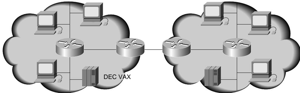
DECnet Phase IV is the most widely implemented version of DECnet. However, DECnet/OSI is the most recent release. DECnet Phase IV is based on the Phase IV Digital Network Architecture (DNA), and it supports proprietary Digital protocols and other proprietary and standard protocols. DECnet Phase IV is backward compatible with DECnet Phase III, the version that preceded it.
