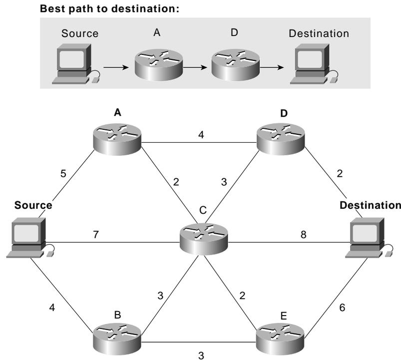
DECnet routing decisions are based on cost, an arbitrary measure assigned by network administrators to be used in comparing various paths through an internetwork environment. Costs typically are based on hop count or media bandwidth, among other measures. The lower the cost, the better the path. When network faults occur, the DRP uses cost values to recalculate the best paths to each destination.
