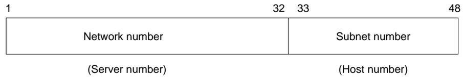
The network number identifies a VINES logical network, which is represented as a two-level tree with the root at a service node. Service nodes, which are usually servers, provide address resolution and routing services to clients, which represent the leaves of the tree. The service node assigns Vines Internetwork Protocol (VIP) addresses to clients.
