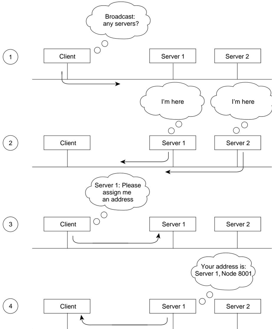
Dynamic address assignment is not unique in the industry (AppleTalk also uses this process), but it certainly is not as common as static address assignment. Because addresses are chosen exclusively by a particular server (whose address is unique as a result of the hardware key), very little chance exists for duplicating an address. This is fortunate because duplicate addresses could cause potentially devastating problems for Internet Protocol (IP) and other networks.
