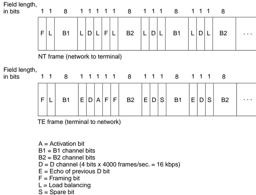
Multiple ISDN user devices can be physically attached to one circuit. In this configuration, collisions can result if two terminals transmit simultaneously. Therefore, ISDN provides features to determine link contention. When an NT receives a D bit from the TE, it echoes back the bit in the next E-bit position. The TE expects the next E bit to be the same as its last transmitted D bit.
