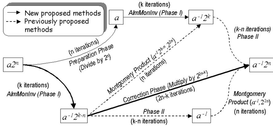
**Fig. 3 Different ways to compute the Montgomery inversion**
