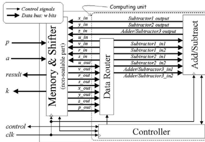
**Fig. 4 Improved inversion scalable hardware block diagram**
