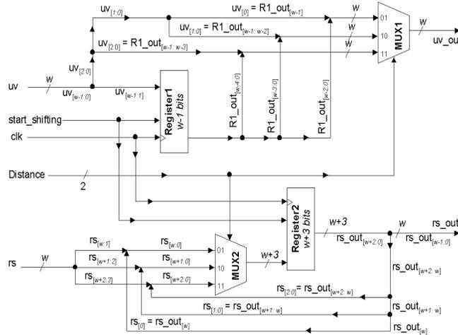
**Fig. 2 Multi-bit shifter (max distance = 3)**
