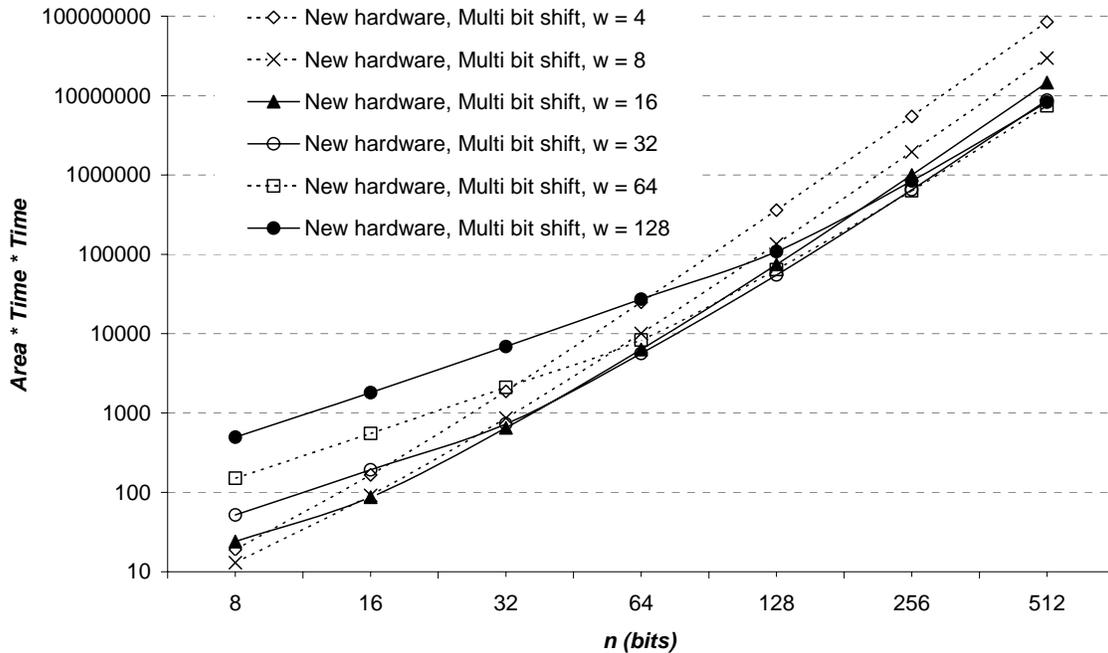
**Fig. 13 Area $\times$ Time<sup>2</sup> figure of merit of different new hardware multi bit shifting architectures**
