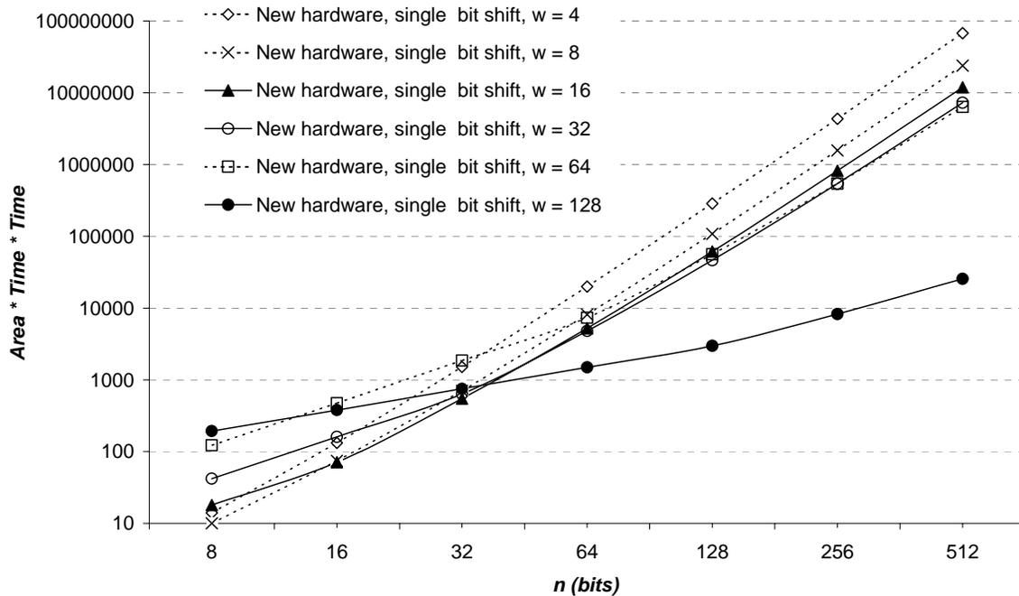
**Fig. 12 Area $\times$ Time<sup>2</sup> figure of merit of different new hardware single bit shifting architectures**
