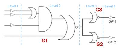
$\rightarrow$  4 Logic Levels  $\rightarrow$  28 Transistors ; Original Circuit had 4 Logic Levels
