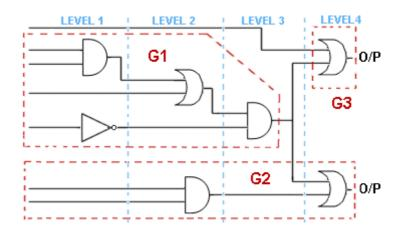
Starting from Logic Level One (the closest to the I/Ps), convert into CMOS using the following logic transformations:
