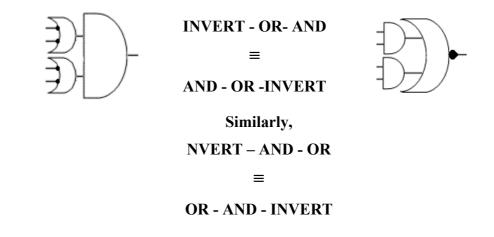
S<sup>rd</sup>. Gates are converted by inserting <u>Bubbles</u>, in pairs, either at the I/Ps or O/Ps & transfer the gates into CMOS.
