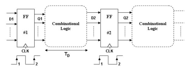
• Based on the FF & combinational logic timing parameters, the following timing constraints are obtained for correct operation of the circuit:
