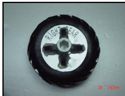
Figure 15: Four magnets fix on the back wheel.
