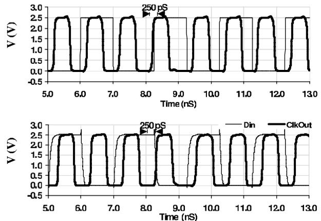
Fig. 9 Simulation results of the NRZ input and output clock of the CRC @ 1 Gb/s. An input phase error of 250 pS is injected and the CRC immediately retimes the output clock.
