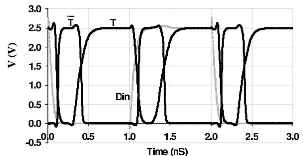
Fig. 3 Simulation of the input/outputs of the DED circuit.
