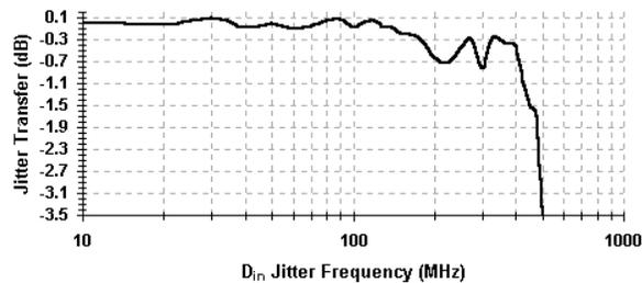
Fig. 15 The jitter transfer characteristics of the proposed CRC for a 1 UI peak-to-peak input data jitter and as a function of jitter frequency.
