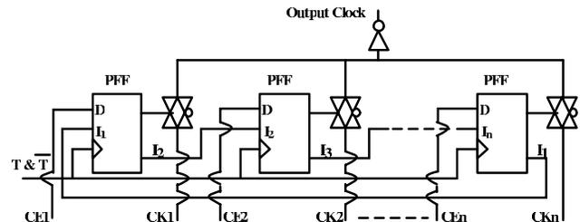
Fig. 6 The ELCM circuit's schematic.
