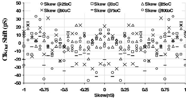
Fig. 10 Shifts in output clock edge relative to Din versus skew between Din and CK<sub>in</sub> for several temperatures.
