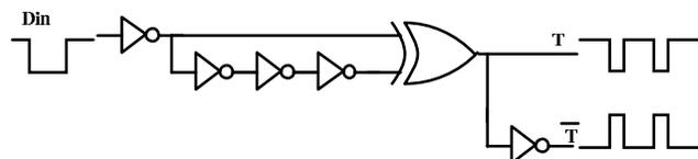
Fig. 2 The double-edge detector circuitry.
