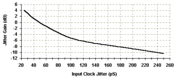
Fig. 14 The CRC's output/input clock jitter gain in dBs.
