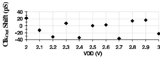
Fig. 11 Shifts in Clk<sub>Out</sub> edge relative to Din vs. VDD.
