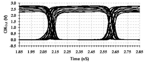
Fig. 12 The output clock jitter with a ±0.25 V and 100 MHz noise superimposed on the supply.
