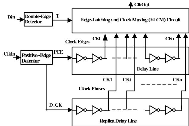
Fig. 1 The architecture of the proposed all-digital CRC.
