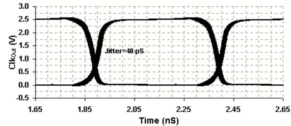
Fig. 13 The CRC's input & output clock jitters.
