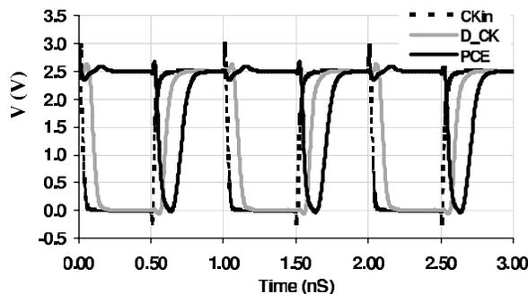
Fig. 5 Simulation results for the PED circuit.
