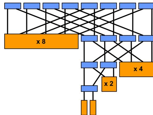
Figure 6 – Trimmed FT Network with Heterogeneous Bandwidth Requirements
