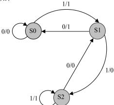
(i) Implement the sequential circuit using D-FFs and the smallest number of gates possible assuming the state assignment: S0=00, S1=01, and S2=10.
