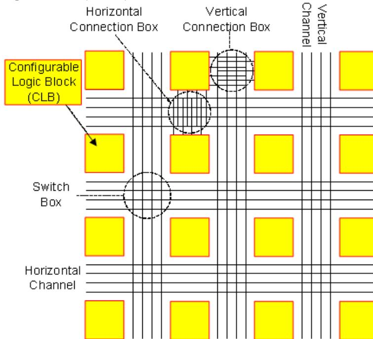
Each CLB can be configured (programmed) to implement *any* Boolean function of its input variables. Typically CLBs have between 4-6 input variables. Functions of larger number of variables are implemented using more than one CLB.
