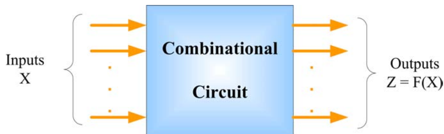
Figure 1: General Block Diagram of a Combinational Circuit
