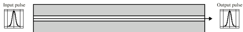
(c) Single mode One path for signal – superior signal quality Used for long-haul telephone and TV comm
