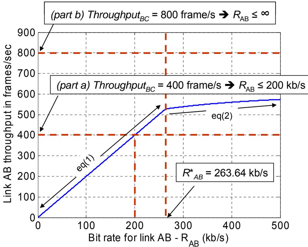
**Figure 1:** Link AB throughput in frames per second as a function of the link bit rate  $R_{AB}$  (kb/s).
