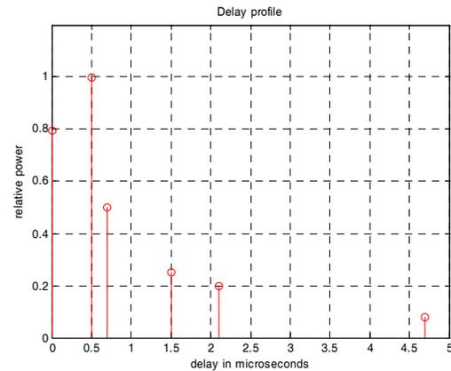
The channel multipath profile is as shown in figure above.
