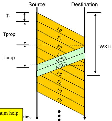
Sending ACK0 as soon as F0 is received is the maximum help the destination can do to increase utilization
