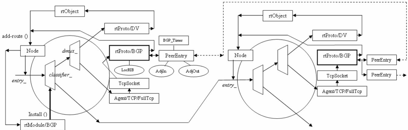
**Figure 2.** Unicast structure of ns-BGP. *rtModule/BGP* manages *classifier\_*. *TcpSocket* resides on top of *Agent/TCP/FullTcp*, while routing protocol *rtProto/BGP* is introduced on top of *TcpSocket*. *rtProto/BGP* has one *PeerEntry* for each peer.
