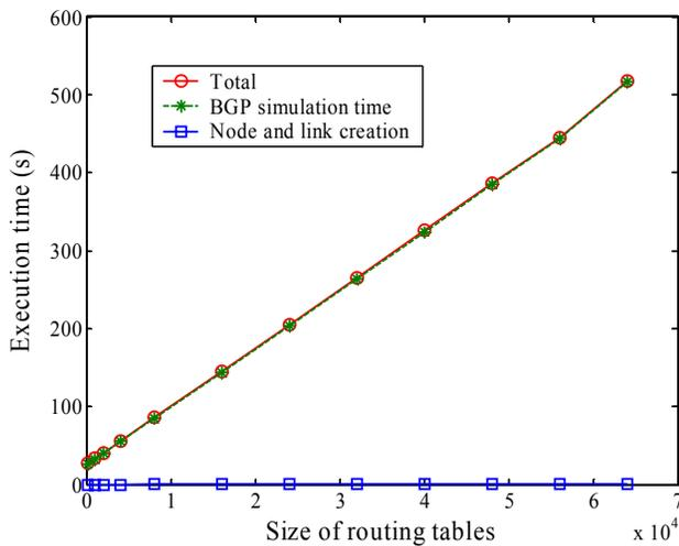
**Figure 6.** Execution time for various sizes of routing tables. Simulated time is 100,000 s. BGP timer intervals are default values as suggested in RFC 1771 [7].
