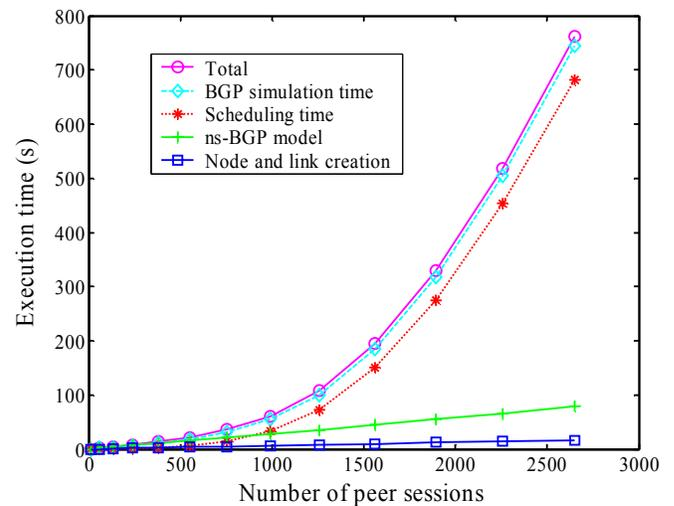
**Figure 5.** Execution times for completely connected networks. Simulated time is 100 s. BGP timer intervals are the default values suggested in RFC 1771 [7].
