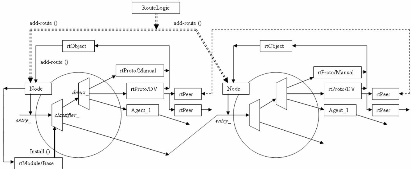
**Figure 1.** ns-2 unicast routing structure. Address classifier (*classifier\_*) and port classifier (*dmux\_*) are two types of classifiers (trapezoids) in an ns-2 unicast node. *Classifier\_* forwards a packet to the *dmux\_* or sends it to a downstream node. *dmux\_* forwards the packet to the corresponding agent.
