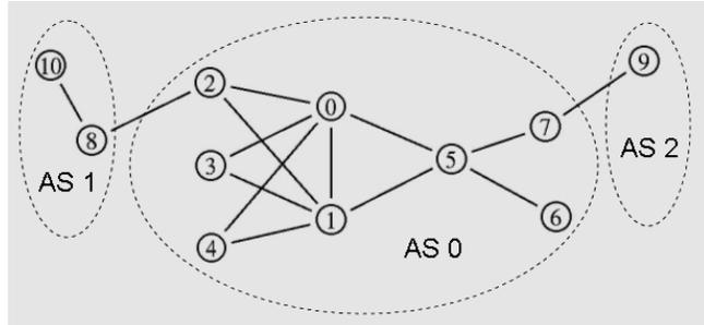
**Figure 3.** Network topology used in the route reflection validation test.
