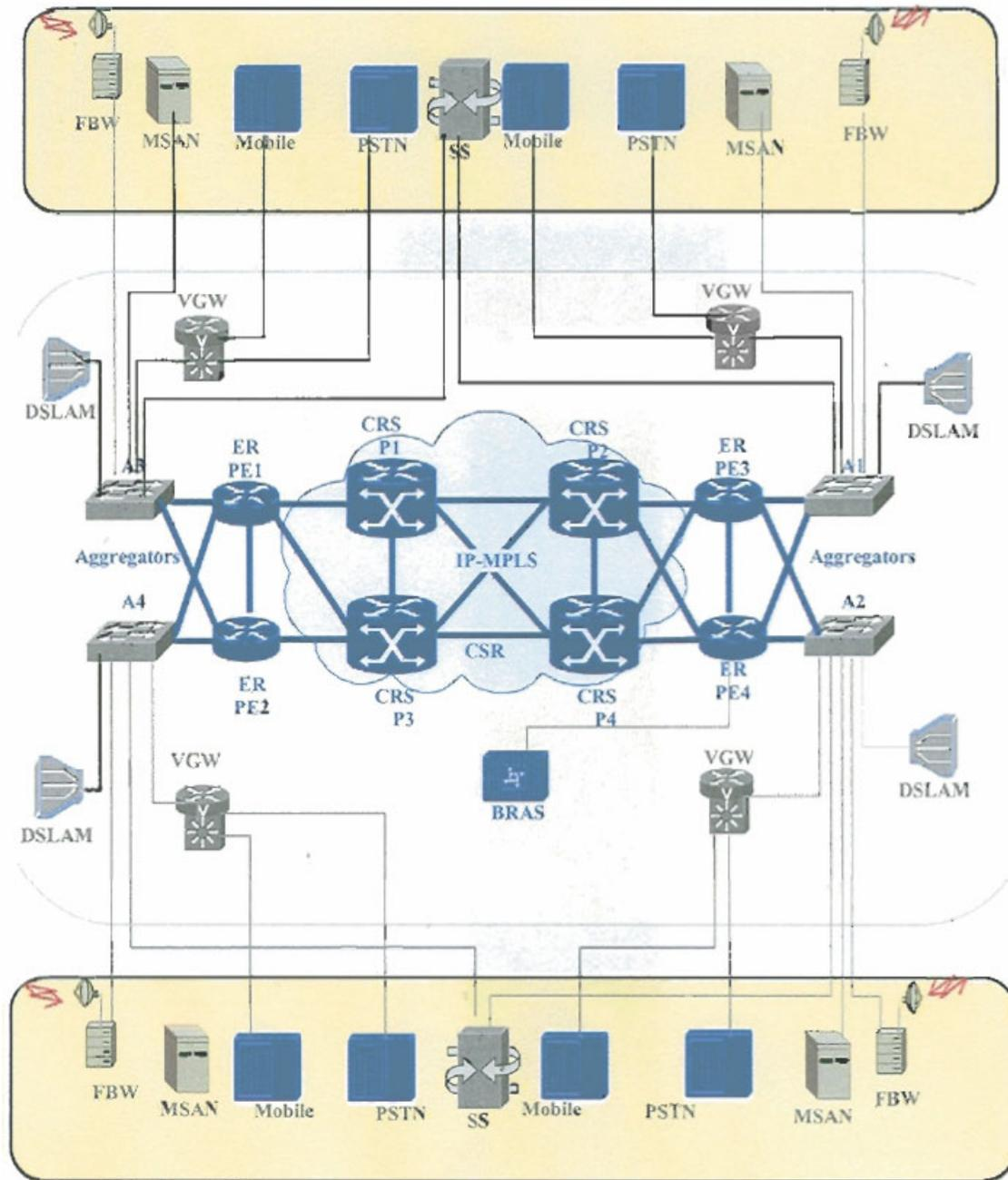
**Fig 1: Service provide core network configuration.**
