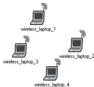
This is an adhoc network of several stations. The workstations can have peer-to-peer connections with other stations in the BSS, but communication is limited to within the BSS.
