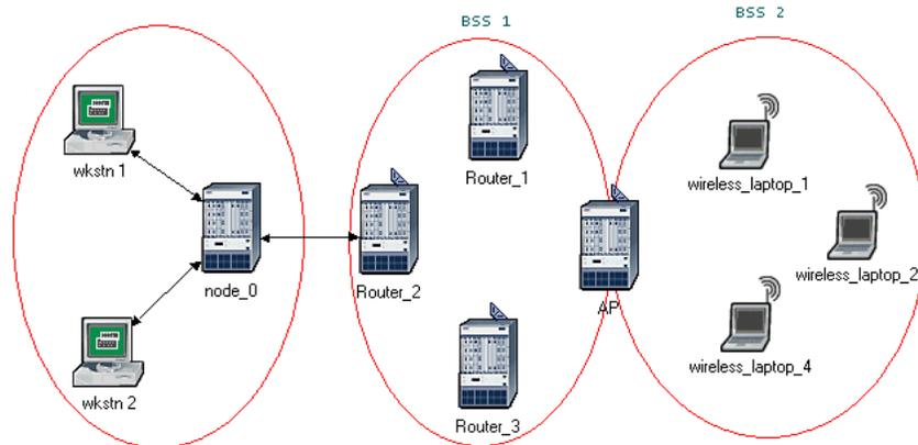
You can set a BSS Identifier for each router interface. Here, Router\_1, Router\_2, Router\_3, and AP form a wireless backbone, BSS 1.
