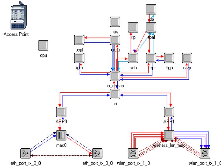
The WLAN router shown in [Figure 9](#) has one wireless interface and one ethernet interface. When it is configured as an access point, which is the default configuration, it can connect a BSS with a wireline distribution system. Do not configure a WLAN interface as an access point if it is part of a WLAN backbone network. When the wireless interface receives a data frame that does not belong to the same BSS, it will send the data frame to the higher layer for address resolution.
