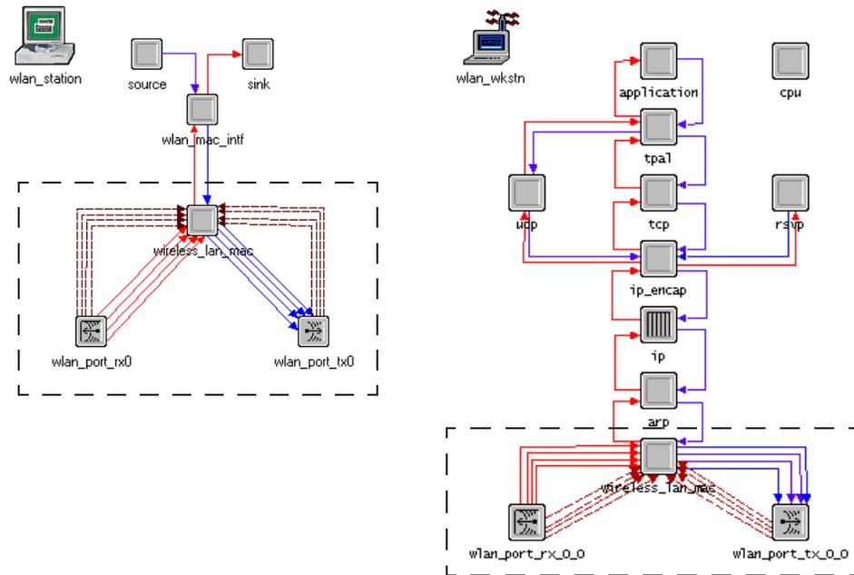
The Wireless LAN modeling of the MAC and the physical layer is comprised of the `wireless_lan_mac` process, transmitter, receiver, and the channel streams (as shown by the box in [Figure 8](#)). The ARP (address resolution protocol) is an interface between the MAC and the higher layers.
