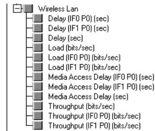
Module statistics are collected on a per station basis. Some of the important statistics available from the WLAN MAC module are:
