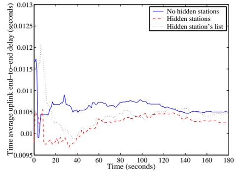
Fig.8 Average uplink end-to-end delay of station 3
