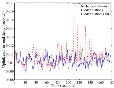
Fig.6 Uplink end-to-end delay versus time
