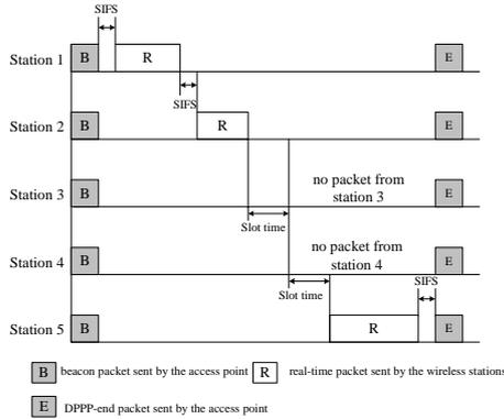
Fig.2 Access procedure of the DPP
