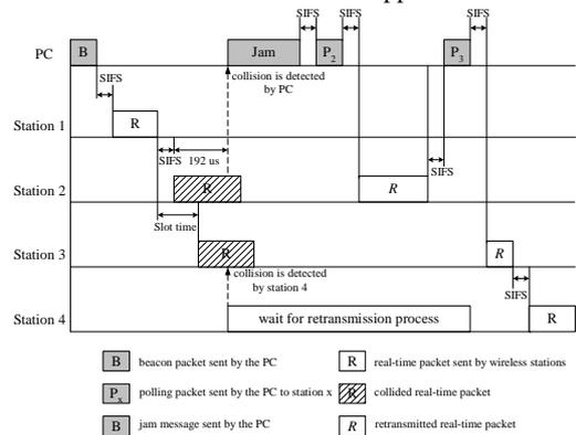
Fig.4 Retransmission process
