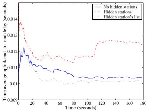
Fig.7 Average uplink end-to-end delay of station 5
