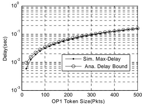
Figure 6. Theoretical delay bound and maximum delay for OP1's flow.
