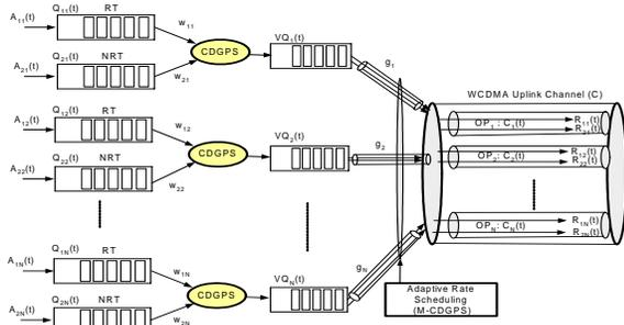
Figure 2. Queuing detail mode for M-CDGPS scheme.
