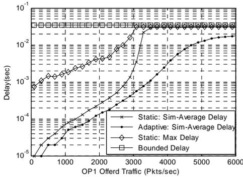
Figure 5. Average, maximum and theoretical bound of OP1's flow delay
