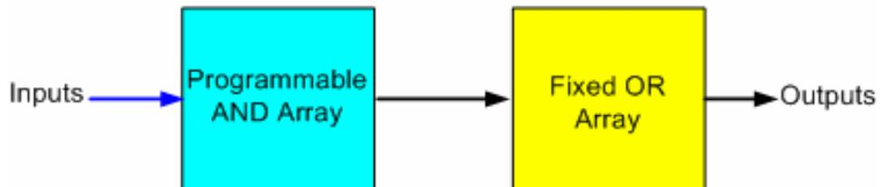
(b) Programmable Array Logic (PAL) Device
