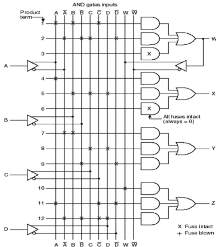
Since both W and X have two product terms, third AND gate is not used. If all the inputs to this AND gate left intact, then its output will always be 0, because it receives both the true and complement of each input variable i.e.,  $AA' = 0$
