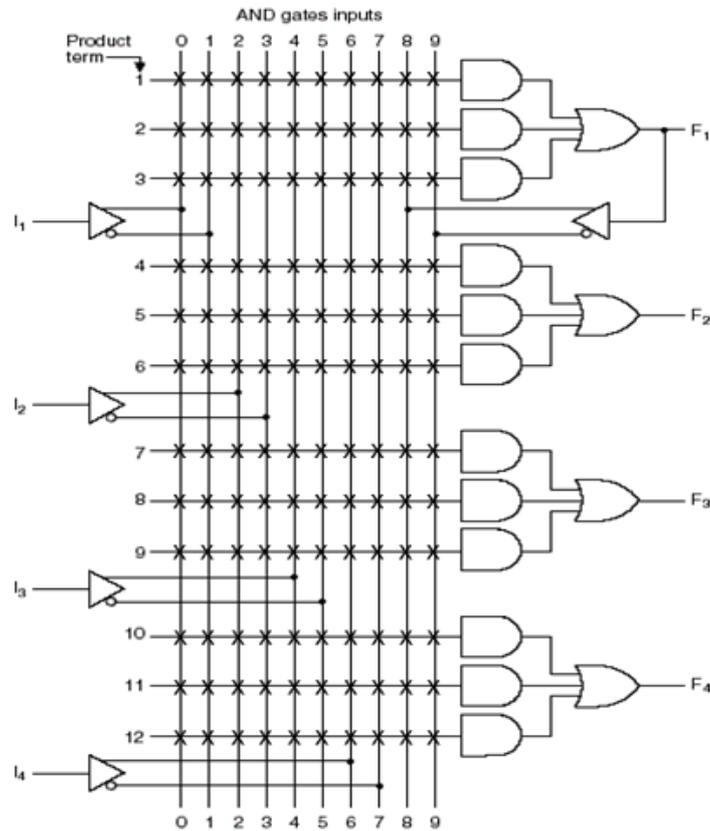
The device shown in the figure has 4 inputs and 4 outputs. Each input has a buffer-inverter gate, and each output is generated by a fixed OR gate.
