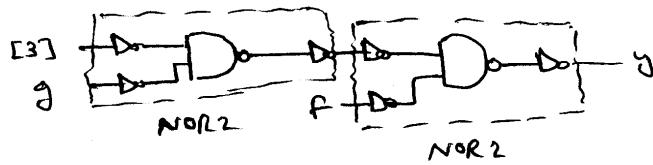
The cost of the fourth graph can be reduced from 19 to 16 by inserting inverter pairs at node [3] as shown below; INV
