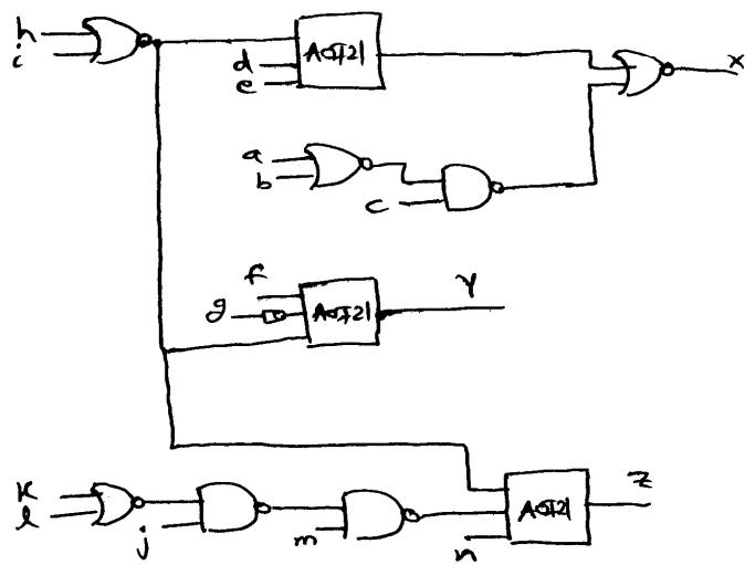
Note that this solution is obtained by taking advantage of inverter optimization across the whole circuit and not just the local subject graphs.
