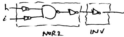
For the third subject graph, inserting two inverters at o14 reduces the cost from 8 to 6 as shown below:
