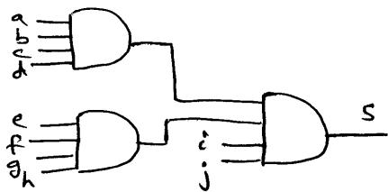
The following decomposition leads to the minimum solution of cost 12
