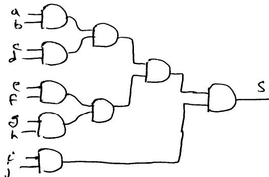
(iii) The pattern trees for the 4-input AND gate cell that need to be stored in the library assuming 2-input AND gates as base functions:
