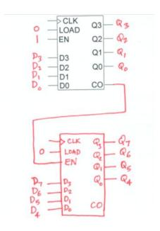
(c) (5 points) Use minimal external gates and the following 8-bit counter to design a counter that counts from 3 to 29 while skipping the counts from 14 to 18 (that is, count from 3 to 13, then from 19 to 29, and then repeat). Assume that the counter is initially loaded with the value 3.
