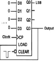
d. Consider the 4-bit feedback shift register shown. Initially the register has the contents ABCD = 1101 and the serial input line is kept at 1. After the arrival of two clock pulses, the register contents
