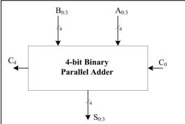
a. Write the Boolean expressions of the  $P_i$ ,  $G_i$ ,  $S_i$  and  $C_{i+1}$  full adder signals. (2 Points)
