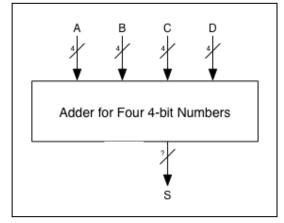
b. Using ONLY 4-bit adders, show how the above circuit can be constructed? [10 pts]
