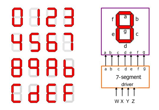
It is required to design a 7-segment display **driver** whose input is a Hexadecimal digit such that the resulting 7-seg display is as shown above (Note that HEX digits larger than 9 are displayed as  $A \rightarrow A$ ,  $B \rightarrow b$ ,  $C \rightarrow C$ ,  $D \rightarrow d$ ,  $E \rightarrow E$ ,  $F \rightarrow F$ ). The driver circuit should generate the 7-segment control signals (a to g).
