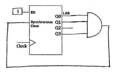
a. Add to the counter the minimum necessary logic required to implement a modulo-12 counter. Indicate all necessary inputs to the counter. (5 points)
