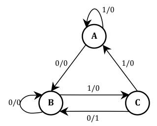
The above figure shows a state diagram of a sequential circuit with one input x and one output y. Trace the state transitions of this circuit by determining the output and the next state given the sequence of inputs and an initial state as shown in the table.
