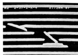
Figure 5: Shorts and breaks of metal lines caused by a scratch in the photoresist.
