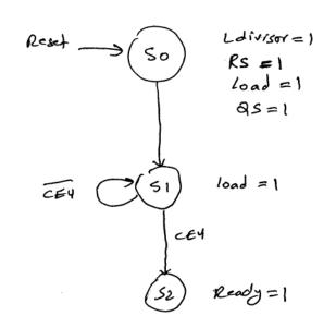
To guarantee correct operation, reset reeds to be synchronous.
