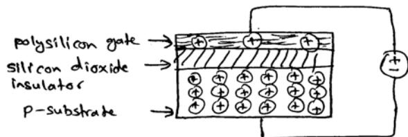
initially, the p-substrate has holes, and when  $V_{GS} \ll V_T$  nothing happens.
