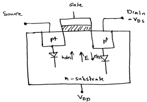
Application of a negative gate voltage (with respect to source) draws holes into the region below the gate resulting in the channel changing from the n-type to the p-type. Thus, a conduction path is created between the source and the drain.
