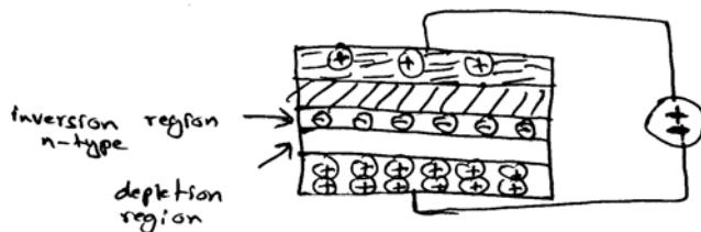
When  $V_{GS}$  is raised further above  $V_T$ , electrons are attracted under the gate. This forms a conductive layer of electrons in the p-substrate.
