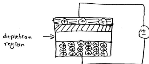
When  $V_{GS}$  is raised above  $V_T$  in potential, the holes are repelled causing a depletion region under the gate.
