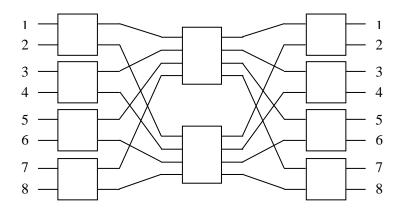
2. Draw a baseline network connecting the 8 processors to the 8 memory modules, and illustrate its routing strategy. Explain how the routing strategy can be used to connect processor 2 to memory module 3.
