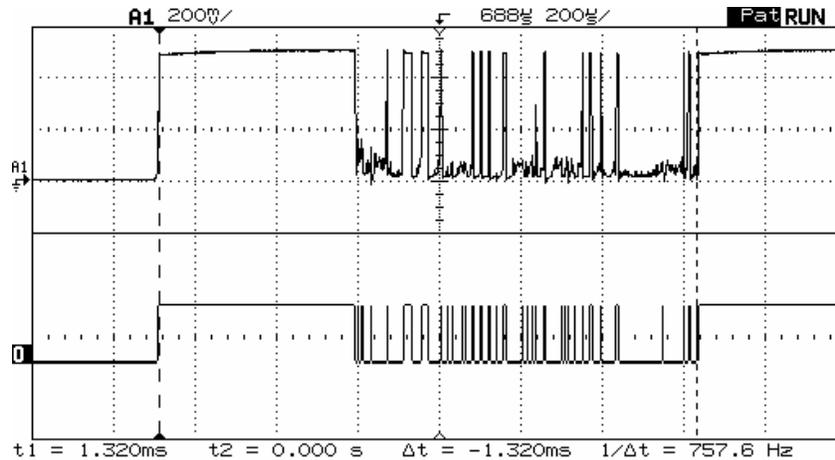
*Switch Q – when released, it goes high for 480  $\mu$ sec before generating 840  $\mu$ sec of hash, a sure way to blow an interrupt system mad if poorly designed.*
