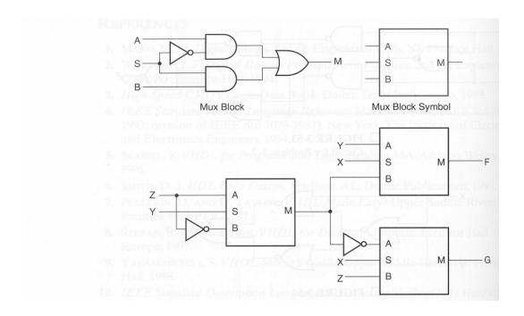
**Q.3.** Find the truth table for the outputs F and G of the hierarchical circuit shown below.
