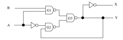
(i) Draw the timing diagram for the outputs X and Y given the waveforms for the inputs A and B shown below. Assume that Y is initially having the value 0.
