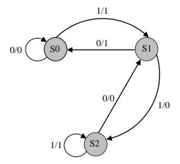
Implement the sequential circuit using JK-FFs and the smallest number of gates possible assuming the state assignment: S0=00, S1=01, and S2=10. Show the state table and minimize your equations using K-map method.
