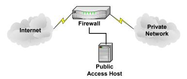
PowerWallz firewall products can be easily deployed using this design because most of the products come with a built in DMZ port for adding a third network. This means no additional hardware costs or upgrades are required with the PowerWallz products.
