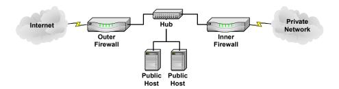
PowerWallz firewall products can be easily deployed using this design because the products utilize the "stealth" technology. This allows the Outer firewall to be completely transparent to the Internet, yet provides the full protection for the Public Hosts and Private Network. By utilizing the "stealth" technology, minimal configuration and management is required to deploy this network design.
