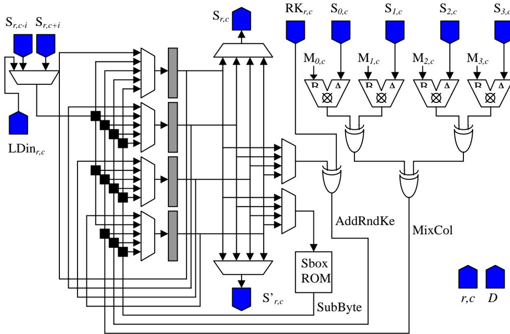
Figure 2 – Byte Datapath Internal Structure
