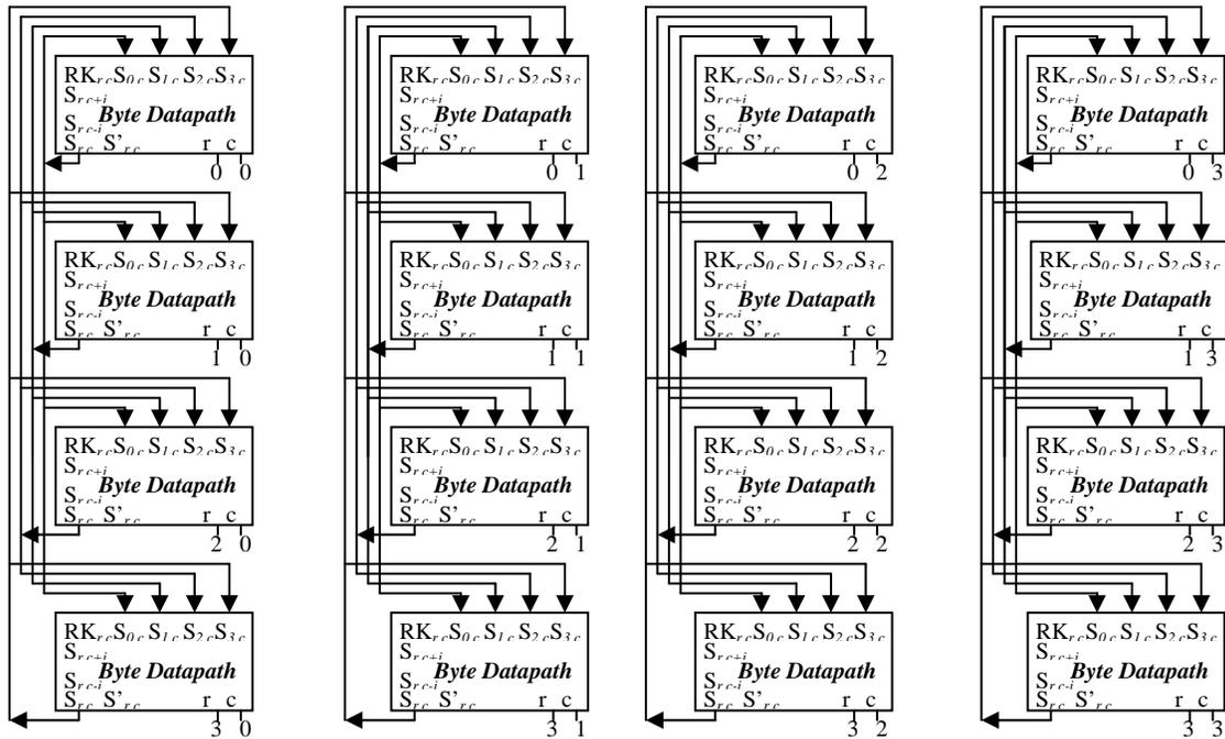
Figure 6 – Mix-Columns Operation Connections
