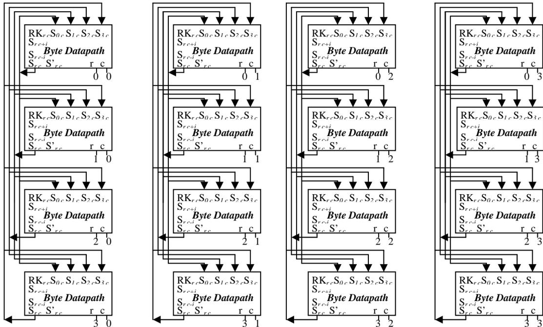
Figure 6 – Mix-Columns Operation Connections
