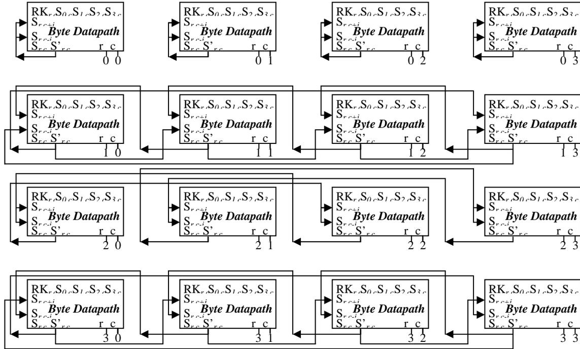
Figure 5 – Shift Rows Operation Connections
