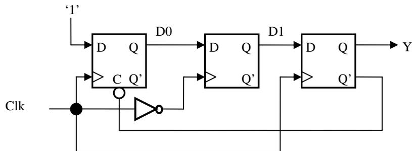
All the flip-flops are positive edge triggered. At initialization, they are all initialized to 0. Draw the timing diagram showing **Clk** and **Y**. You may want to represent any intermediate signal (**D0** or **D1** or both) to help you determine the value of **Y**. The representation of **D0** or **D1** is not mandatory.
