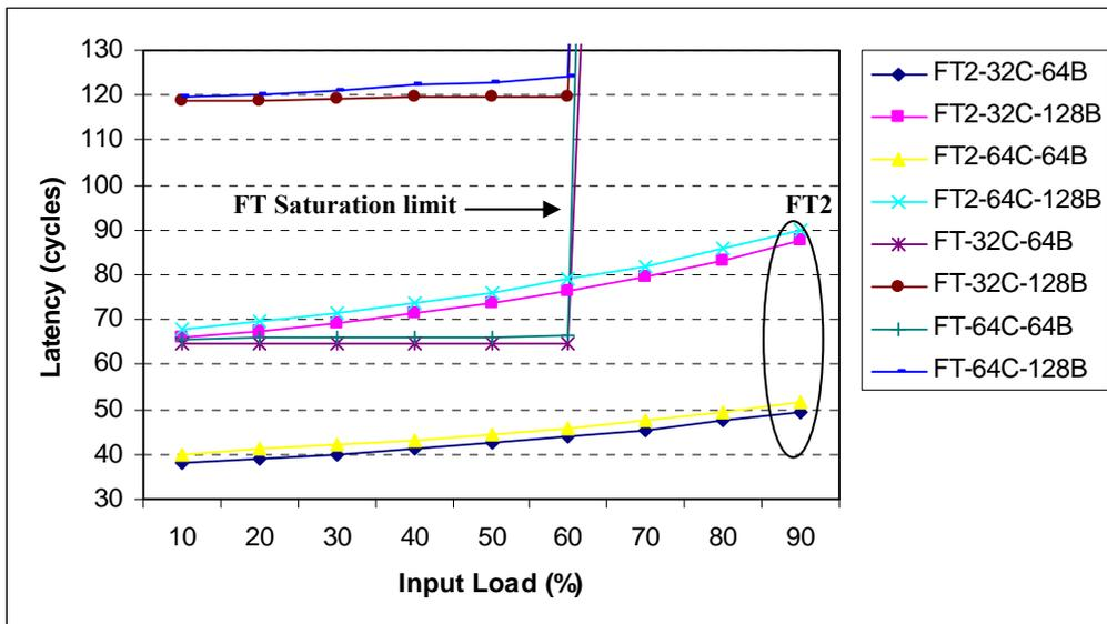
**Figure 11 – Latency versus packet injection rate for regular Fat-Tree (FT) and the modified FT (FT2). Combinations of two network sizes; 32 clients (32C) and 64 clients (64C) and two ranges of packet sizes; 64 bytes (64B) and 128 bytes (128B) were used. The actual packet size within the range was randomly generated (multiples of bytes).**
