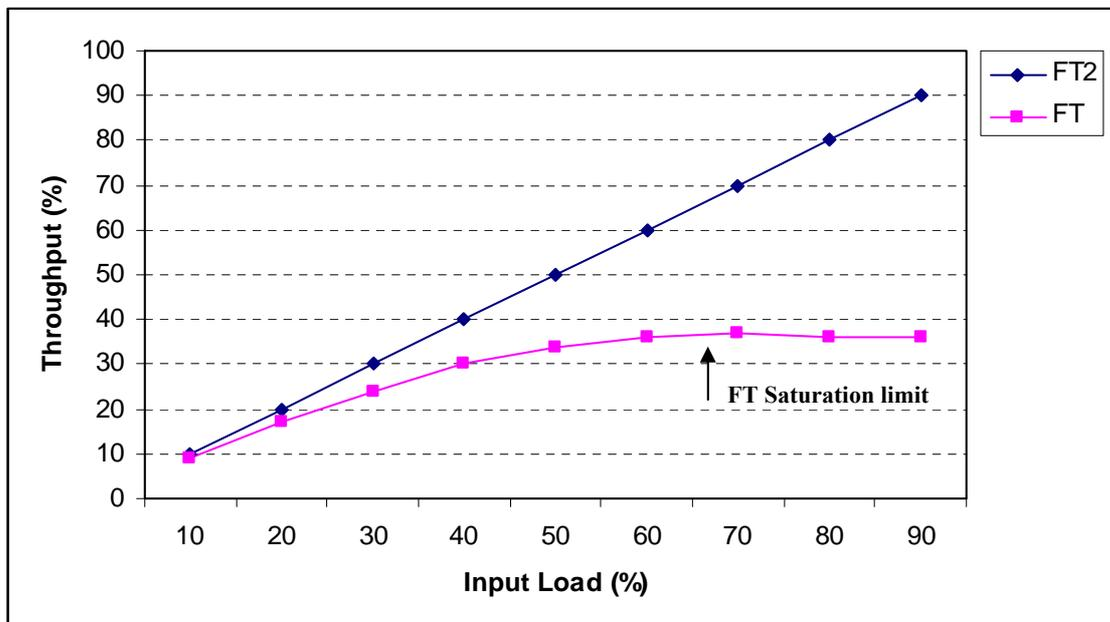
Figure 10 – Throughput versus packet injection rate for regular Fat-Tree (FT) and the modified FT (FT2).
