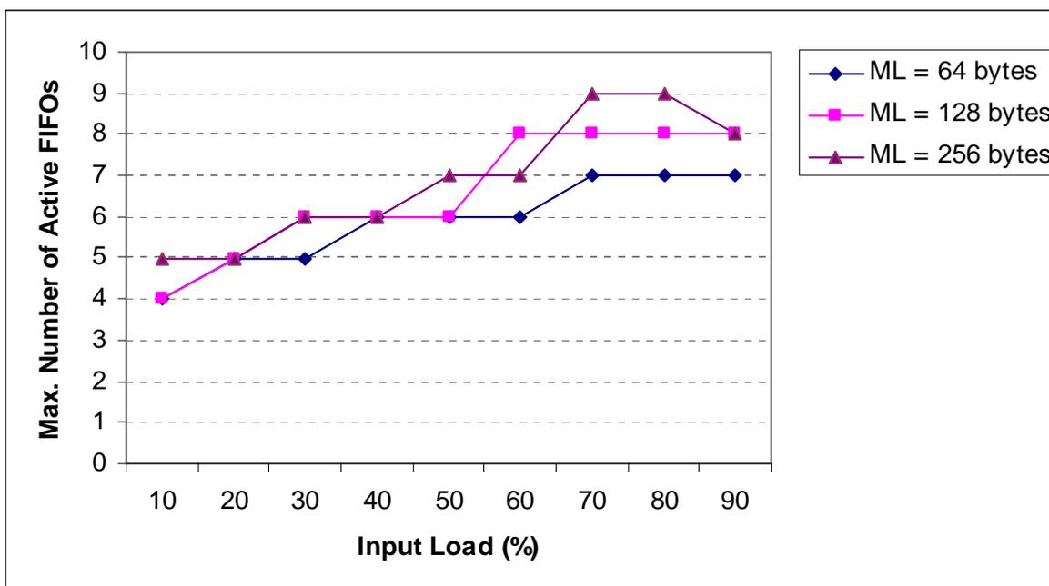
Figure 13 – Maximum number of FIFO lanes simultaneously active per client versus injection rate for several packet sizes (ML).
