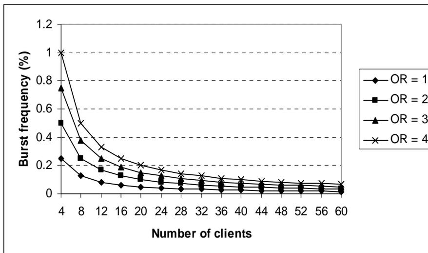
Figure 12 – Maximum burst frequency as a function of the number of sending clients in the burst for several FIFO emptying rates.
